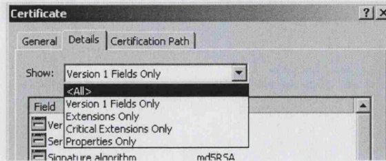
Figure 5 - An illustration of a certificate listing most of the fields in X.509 Version 3
