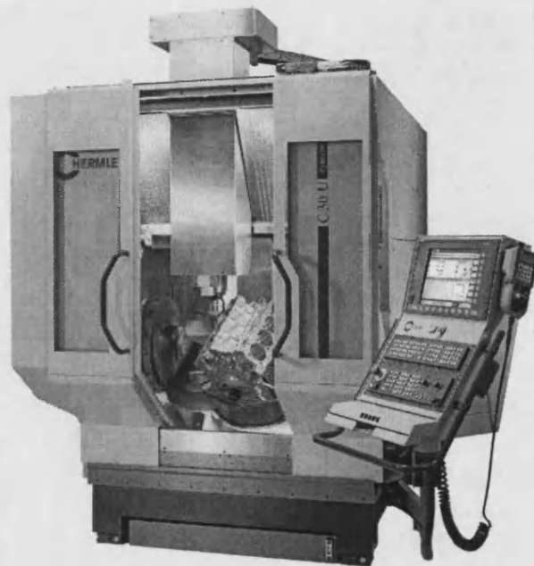
Figure 4.5: CNC (computer numerical control) machine used in production of moulds (2006)
