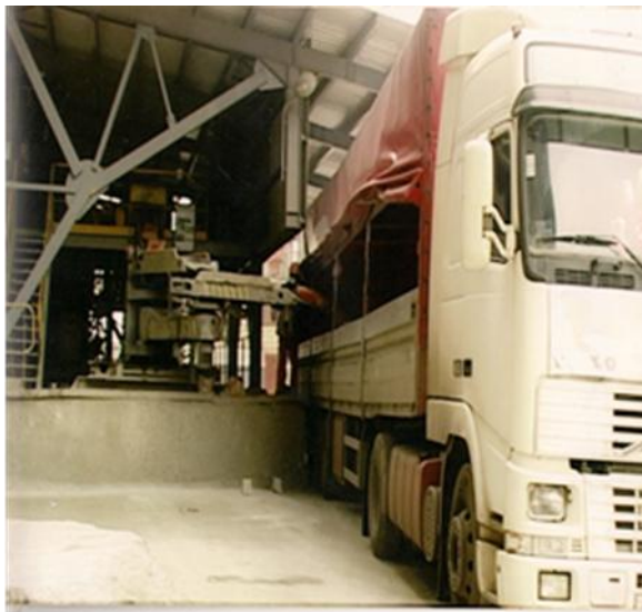
Figure 30. Mechanical cement-bag loading at the Distribution Centre of Ciment S.A. (Courtesy of Ciment S.A.)
