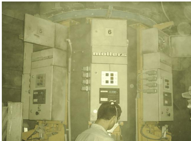
Figure 20. Automated cement packaging at the Rybnitsa Cement Plant.
