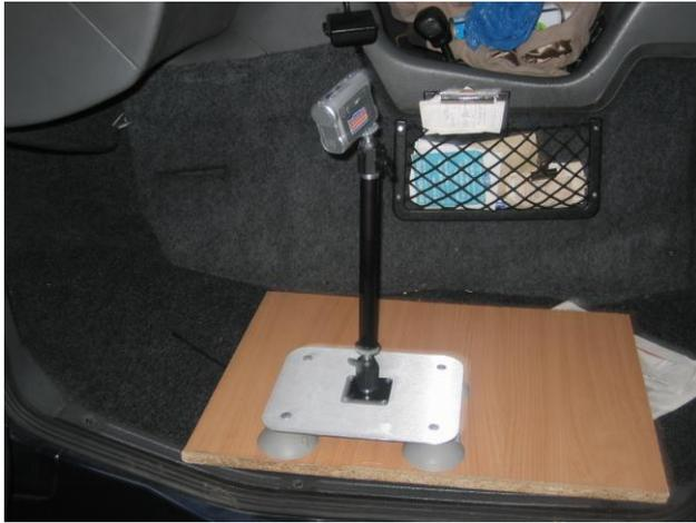
Figure 4.3: Sticky Pod and Camera Mounted in Black Cab Floor next to Driver Seat
