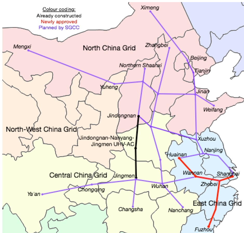
Figure 6.2 UHV-AC project approvals in the East China Grid (2011-2013) Author's visualisation of material presented in this section.
