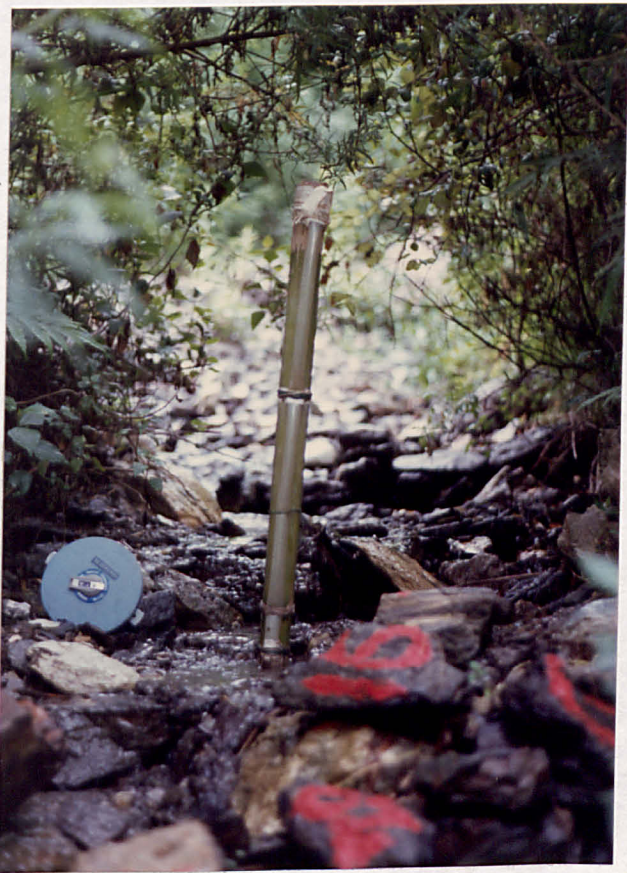
FIGURE 8.2 and PLATE 8.1 The Crest-Stage Recorder
