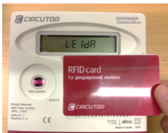
FIGURE 2 METER ACTIVATION. THE PREPAID CARD IS USED TO TOP-UP THE METER EACH TIME THE HOUSEHOLD RUNS OUT OF CREDIT
