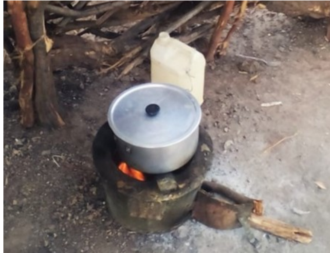
Figure C.4: Example of portable improved cookstove (ICS) fuelled with firewood, Kakuma. Source: Practical Action, Moving Energy Initiative.
