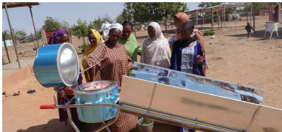
Figure C.5: Example of Blazing Tube (solar cooker) trialled in Saag-Nioniogo Camp, Burkina Faso. The same model was also trialled in Goudoubo. Source: UNHCR via Clean Cooking Alliance; accessed on February 10, 2020 at the link: https://www.cleancookingalliance.org/about/news/10-20-2015-blazing-tube-solar-cookers-in-burkina-faso-refugee-camps.html .
