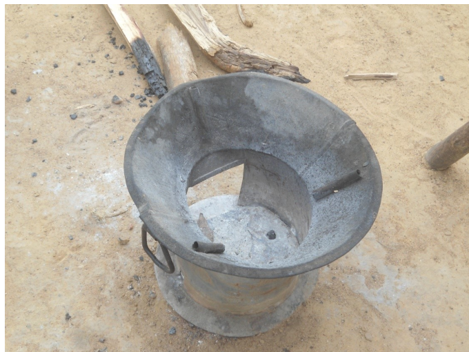
Figure C.3: Example of metallic portable improved cookstove (ICS) fuelled with firewood, manufactured by blacksmiths in Goudoubo. Source: Practical Action, Moving Energy Initiative.
