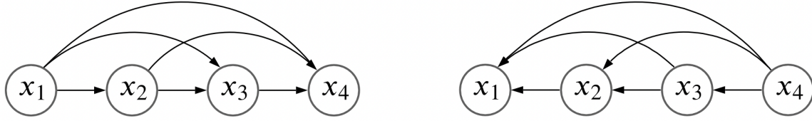
Fig. 2.2 Diagrams showing two different autoregressive models defined by different orderings of the variables.
