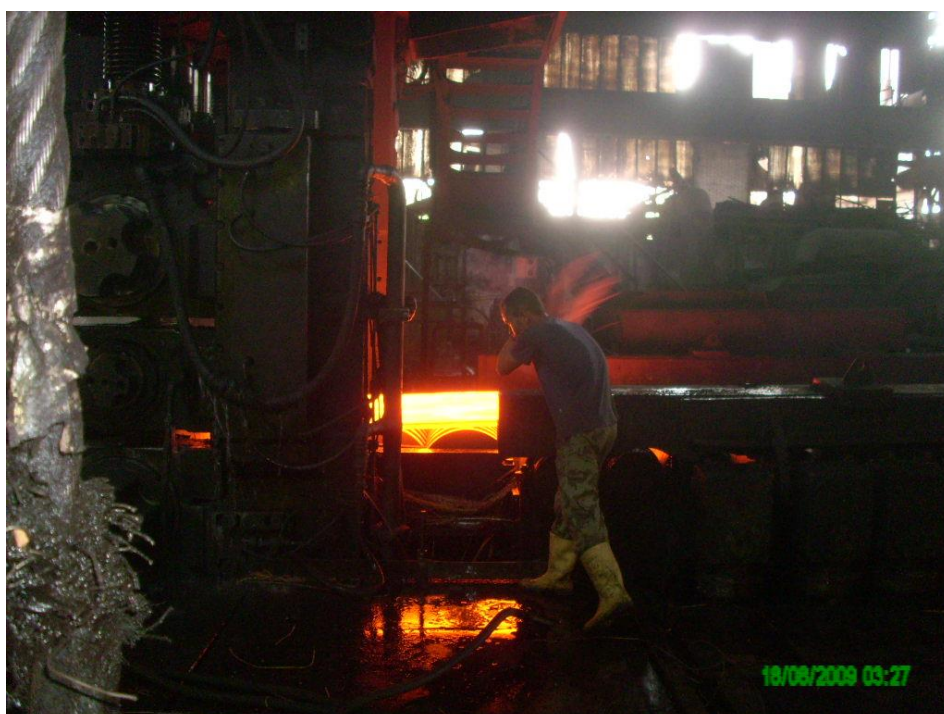
Figure 17: Using Chaff to Clear Oxides from the Slab
