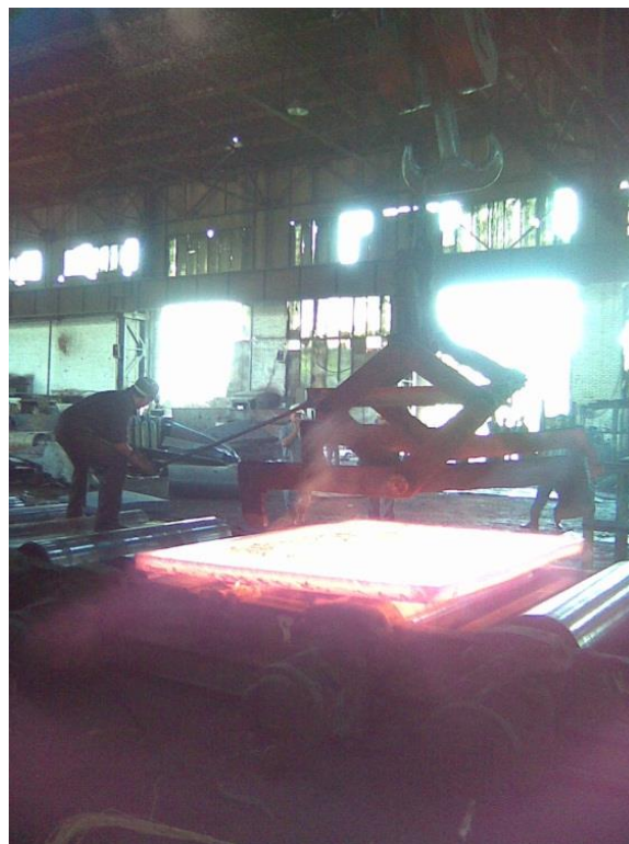
Figure 19: Fadi Assists the Crane Operator with Crowbar to Attach the Sheaves
