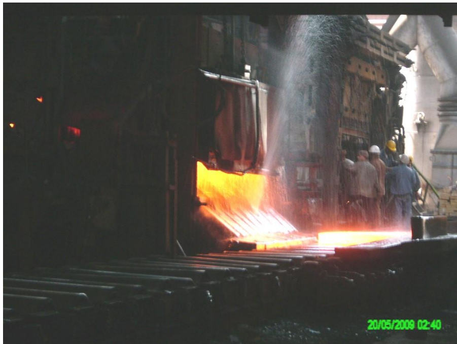
Figure 8: Steel Slab Released From Re-heating Furnace
