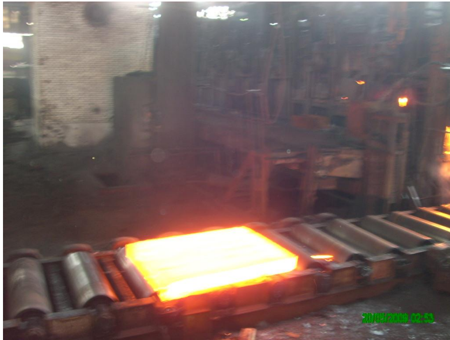
Figure 9: Slab Slides on Rollers towards 3-High Rolling Mill
